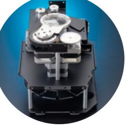
▲ Rotating three-facet prism and high-speed dual-blade shutter provides 1-7 Hz strobe effect.
