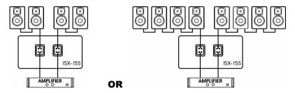
**ISX-10**: You can connect up to 2 "ISX-10" cabinets to each subwoofer output. This means a total maximum of 4 cabinets. (see drawings)
