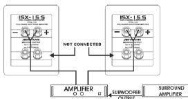
out" from your surround sound amplifier. In this setup the ISX-15S subwoofer will act as a mono subwoofer. This means it must be connected in a different way: don't use the outputs and connect the subwoofer as shown on the drawing.
