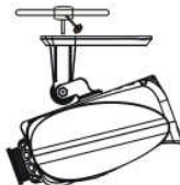
montage in truss
