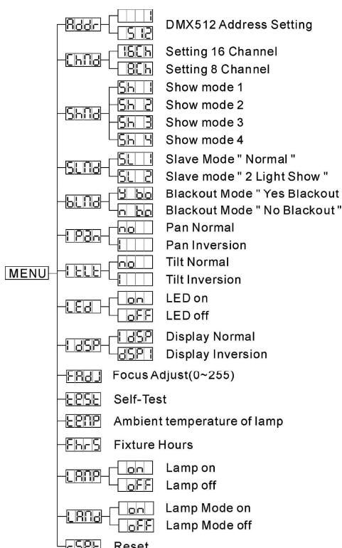
**Sh 1** Show 1 mode- Fixture is placed **on the floor**. Tilt movement angle 210°.**Sh 2** Show 2 mode-Fixture is fixed **under ceiling**. Tilt movement angle 90°.**Sh 3** Show 3 mode - Fixture is placed **on a podium, in front of the audience**
