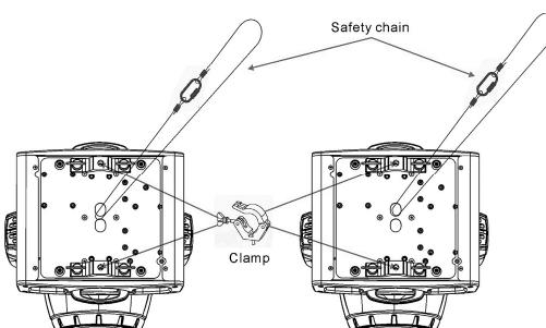
away from any flammable materials and/or liquids. The fixture must be fixed at least 50cm from surrounding walls.
