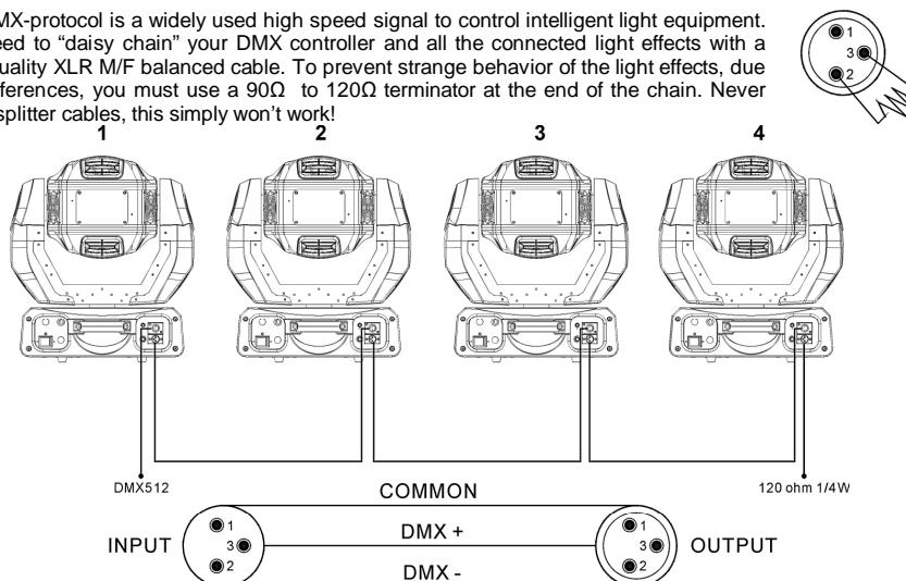
Each light effect in the chain needs to have its proper starting address so it knows which commands from the controller it has to decode.
