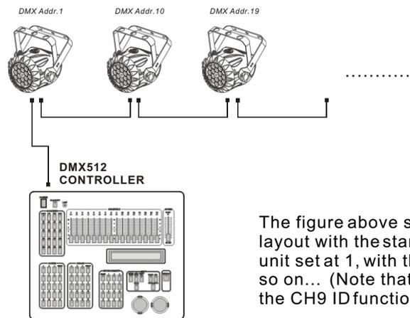
The figure above shows a simple DMX512 layout with the starting address of the first unit set at 1, with the second set at 10 and so on... (Note that when used in this way, the CH9 ID function must be inactive (CH9=0))
