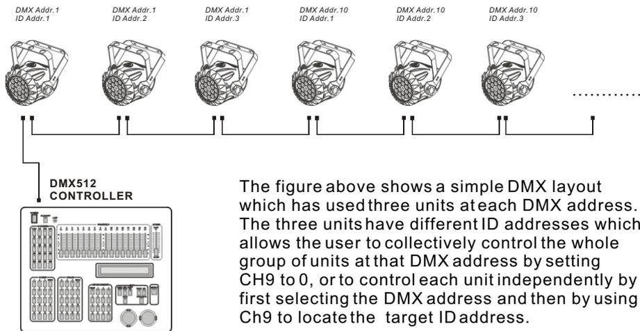
The figure above shows a simple DMX layout which has used three units at each DMX address. The three units have different ID addresses which allows the user to collectively control the whole group of units at that DMX address by setting CH9 to 0, or to control each unit independently by first selecting the DMX address and then by using Ch9 to locate the target ID address.
