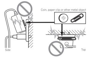
The power plug could come detached from the AC adapter and remain in the power outlet if someone trips on the AC adapter's power cord or if something hits the AC adapter. If this happens, remove the power plug remaining in the outlet with dry hands, holding it as shown on the diagram below and without touching metal parts. Do not use any tools to remove it.
