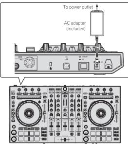
7 Press the [STANDBY/ON] switch on this unit's rear panel to turn this unit's power on.
