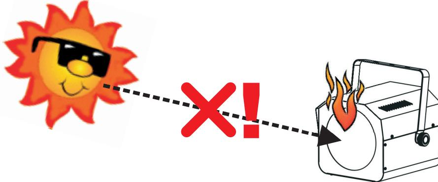
**WARNING: DANGER!** never expose the lens to direct sunlight, even for a short period. This may damage the light effect or even cause fire!
