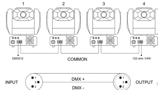
Each light effect in the chain needs to have its proper starting address so it knows which commands from the controller it has to decode.
