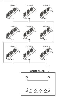
In the figure above the PiX controller is connected in series to 9 units with corresponding ID addresses from 1 to 9. Each fixture has **[ID ON]** in the fixture's **[Settings]** menu. In order to activate the **[Effect]** programs in the PIX CONTROLLER, the **[Range]** must be set to **[009]** in the **[Settings]** menu of the PIX CONTROLLER. (Note: it is possible to create different kinds of effects by changing the direction and position of ID Addresses)
