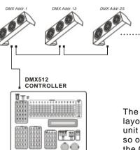
The figure above shows a simple DMX512 layout with the starting address of the first unit set at 1, with the second set at 13 and so on... (Note that when used in this way, the CH10 ID function must be inactive (CH10=0))
