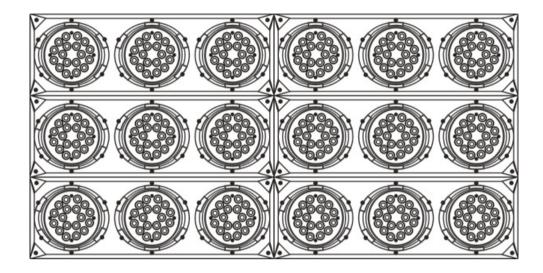
The 'male' and 'female' connections enable the fixtures to be interlocked together in the way shown in the diagram. Please note that when multiple units are mounted together it is not necessary to attach every single unit to the truss, wall or weight supporting system. However, it is important to ensure that all fixtures are securely locked together and that each fixture is secured using a safety cable.
