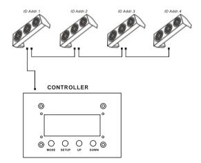
In the figure above the PIX controller is connected in series to 4 units with corresponding ID addresses from 1 to 4. Each fixture has [ID ON] in the fixture's [Settings] menu. In order to activate the [Effect] programs in the PIX CONTROLLER, the [Range] must be set to [004] in the [Settings] menu of the PIX CONTROLLER.
