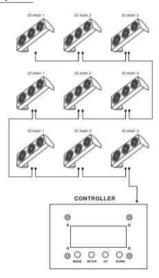
In the figure above the PIX controller is connected in series to 9 fixtures with each row comprising of 3 fixtures with corresponding ID addresses from 1 to 3. Each row is repeated so that the ID addresses appear the same was as the first row. Each fixture has [ID On] in the fixture's [Settings] menu. In order to activate the [Effect] programs in the PIX CONTROLLER, the [Range] must be set to [003] in the [Settings] menu of the PIX CONTROLLER.
